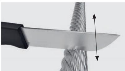
Use a knife to easily detect wire breaks by moving it alongside the rope.
