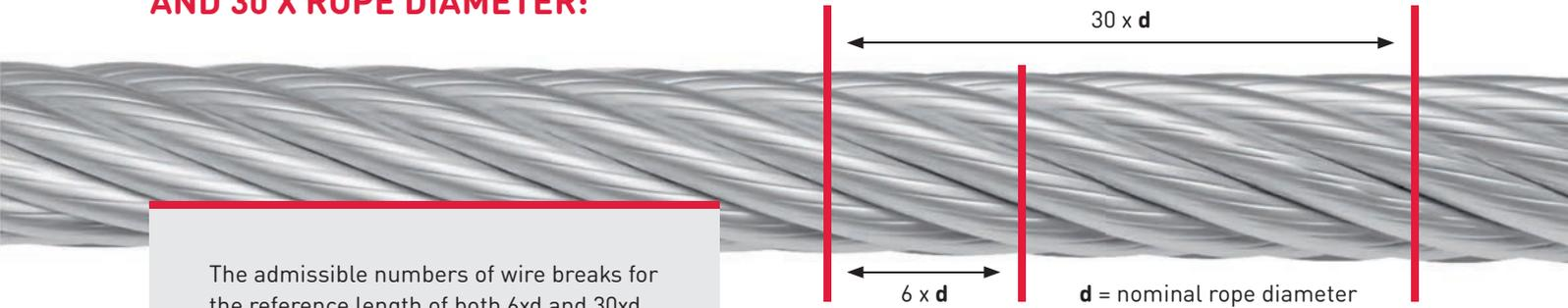
The admissible numbers of wire breaks for the reference length of both 6xd and 30xd are given in the tables on the following pages. The reference sections can be placed independantly and do not need to overlap. If one of these two criteria is met, discard is reached!
