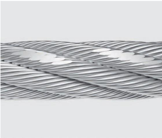
Flattened rope sections are a result of mechanical impact:
