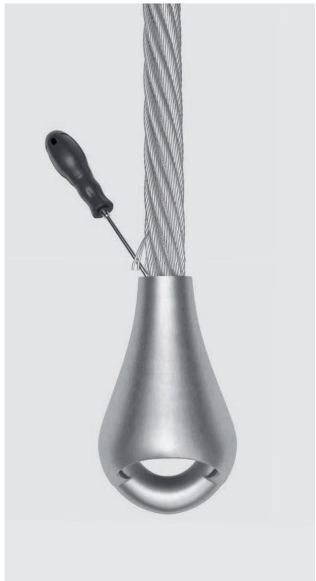
The presence of water may support corrosion which supports the development of wire breaks.
