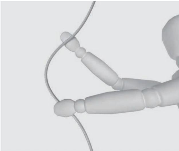
Also, a **seemingly intact** rope can show **lateral wire breaks** when being bent.
