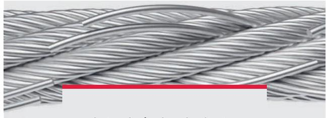
**Lateral wire breaks** due to internal rope wear. **Special attention is required – see page 13!**
