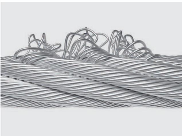
Protruding wires are a result of increased friction within the rope, which hindering the relative sliding movement of the wires.
