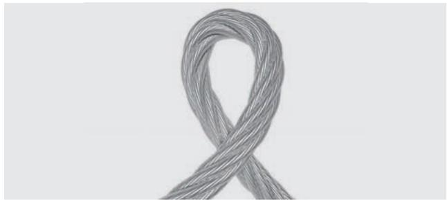
A tightened loop most often is a result of wrong rope handling. Mechanical deformation leads to imbalance of load distribution. Hence rope strength can be reduced seriously.
