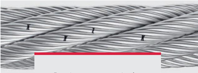
Regular wear: **smooth wire breaks** on the outside due to mere bending fatigue, see the following pages.
