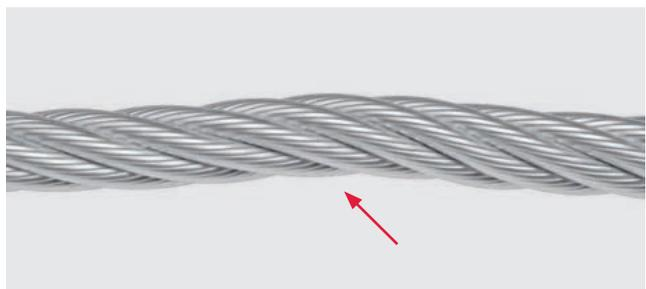
Local diameter decrease most likely is a sign for a broken inner rope element, like a broken rope core. Rope strength is considerably decreased.
