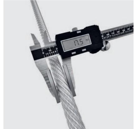
IF THERE IS NO SPECIAL CALIPER AVAILABLE, ENSURE TO MEASURE IN THE CORRECT WAY:
