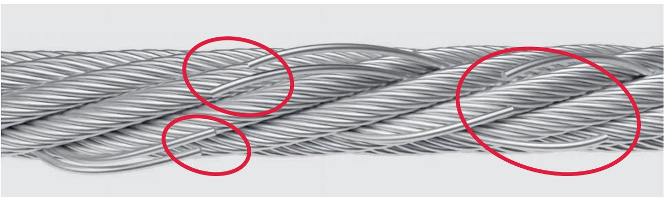
**⚠** If two or more wire breaks in a rope lay length (approx. a length of  $6xd$ ) are present, the rope has to be discarded immediately!
