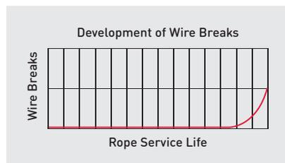
Usually, the increase of bending fatigue wire breaks is not proportional to rope service life, see diagram. **Thus, inspection intervals may be defined according to the recent development of wire breaks.**
