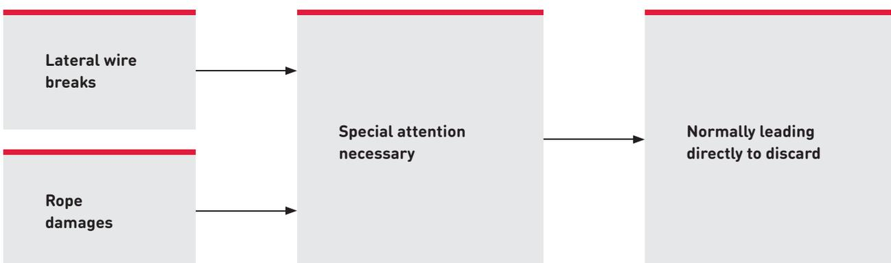
**⚠** The safety of rope drives is highly depending on quality and frequency of rope wear monitoring!
