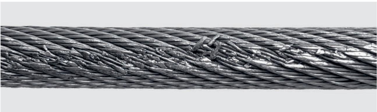
**⚠** For the admissible numbers of wire breaks located in crossing zones, individual limits are existing. See right columns on pages 6 and 7.
