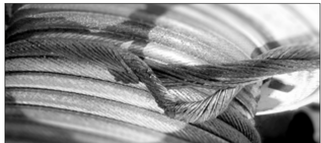
Fig.: Protrusion of the rope core at a non-rotation resistant rope (top) and at a low-rotation rope (bottom)
