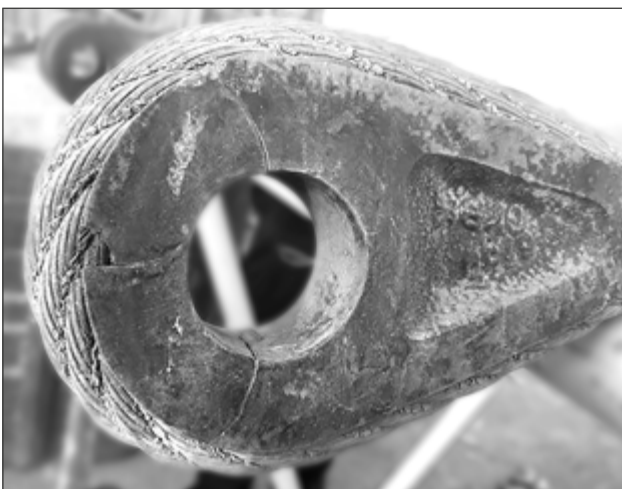
Fig.: Cracks in a solid thimble
