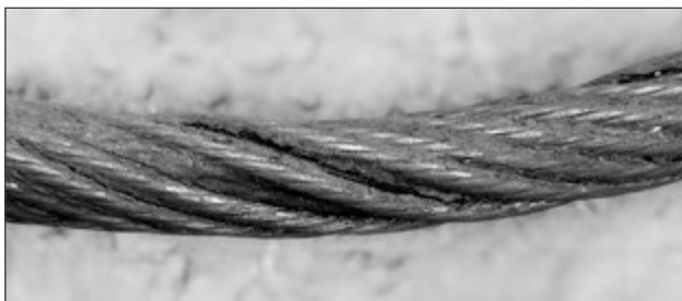
Fig.: Local decrease of rope diameter
