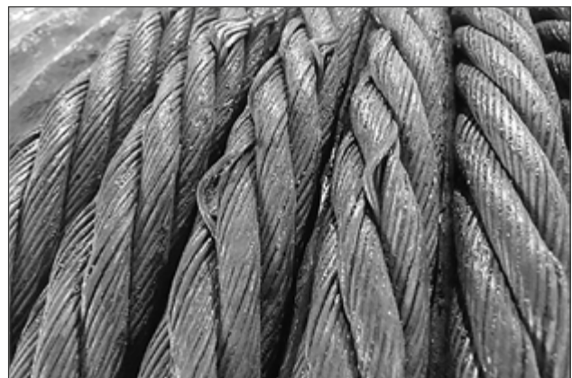
Fig.: Protruding wire loop
