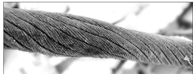
Fig.: Flattened portion
