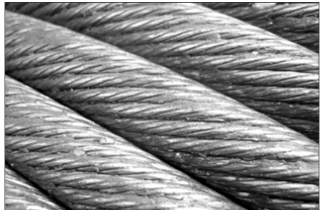
Fig.: Superficial corrosion, rust film
