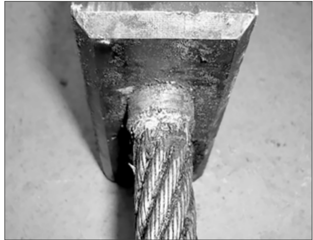
Fig.: Excessive slippage of the socket basket out from the cast socket body
